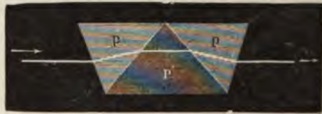
FIG. 53.—Direct-vision prism with three prisms. P , crown; P' , flint.
